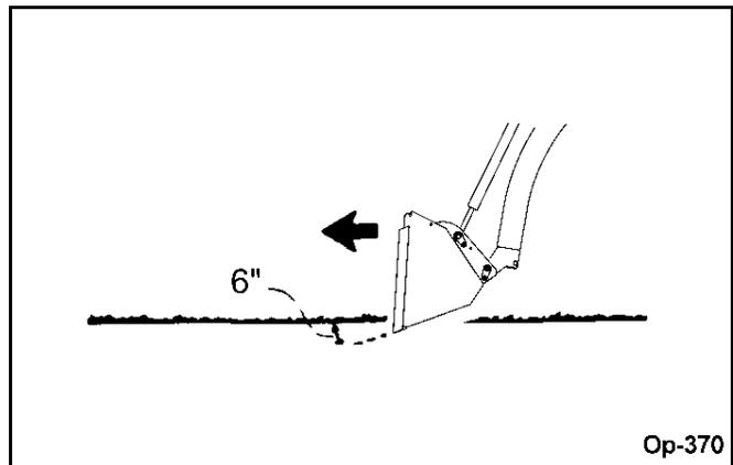
With bucket level, start a cut at notch approximately 2 inches deep. Hold depth by feathering bucket control to adjust cutting lip up or down. When front tires enter the notch, adjust lift cylinder to maintain proper depth.
