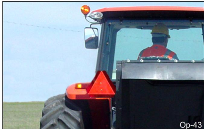
Make sure that all tractor flashing warning lights, headlights, and brake/tail lights are functioning properly before proceeding onto public roads. While newer model tractors have plenty of lighting to provide warning signals and operating lighting, most older models are only equipped with operating lights. Consult an authorized tractor dealer for lighting kits and modifications available to upgrade the lighting on older tractor models. OPS-U- 0021
