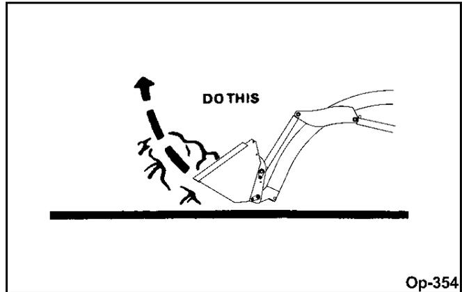
A level bucket throughout the lifting cycle resists bucket lift and increases breakaway effort.
