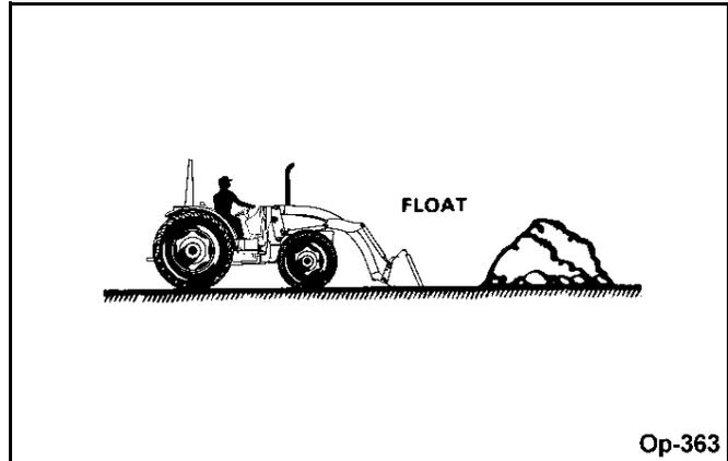
Float will also prevent mixing of surface material with stockpile material. Float position will reduce the chance of surface gouging when removing snow or other material.
