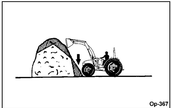
Another method for large dirt piles is to build a ramp approach to the pile.
