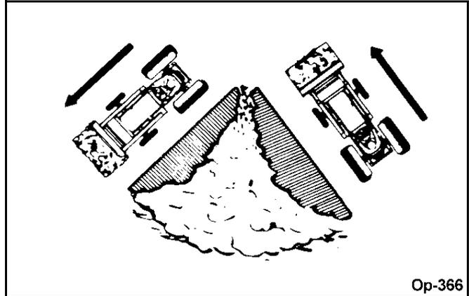
If the pile sides are too high and liable to cause cave-in, use loader to break down the sides until a slot can be cut over the top.
