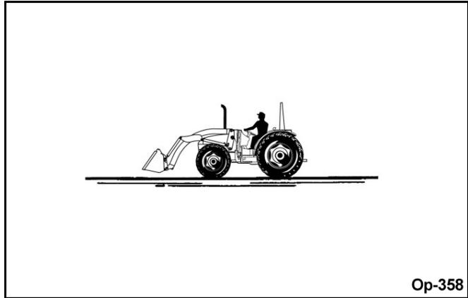
Use extreme care when operating loader on a slope, keep bucket as low as possible. This keeps center of gravity low and will provide maximum stability.
