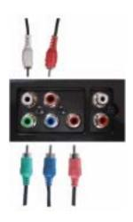
The component connectors split the video signal into three signals, two color and one black-and-white. If you are using the component connectors, you also need to connect the audio cables. To locate the component connectors, see "Bottom View" on page 7.
