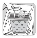
**4.** Clean the rubber seal round the condenser cabinet and in the inner part of the small door with a damp cloth.
