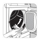
Your dryer will only function well if the filters are clean. The filters collect all the fluff which accumulates during drying and they must therefore be cleaned at the end of each programme, before removing the laundry, with a damp cloth. The light Filter is on to remind you of this operation.
