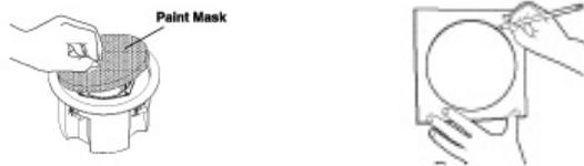
If you choose to paint the speaker frame and grille, use the included cardboard paint mask to protect the speaker. Paint and allow to dry before installing.
