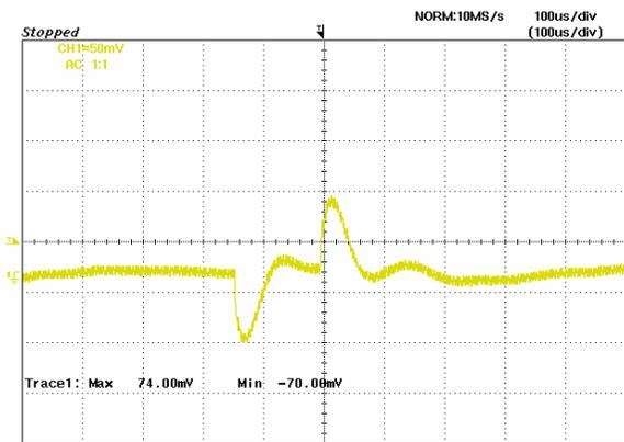
**Figure 21:** Typical transient response to step load change at  $10A/\mu S$  from 50% to 75% and 75% to 50 of  $I_o$ , max at 12Vin, 2.5V out
