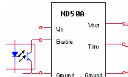
Figure 24: Enable input drive circuit example with isolation.
