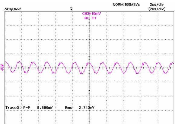
Figure 11: Output ripple & noise at 12Vin, 2.5V/50A out
