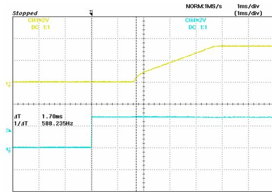
**Figure 16:** Turn on delay time at Remote On/Off, 3.3V/50A out
