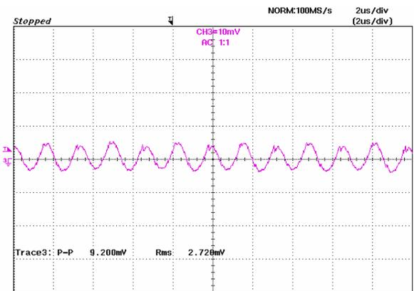
Figure 12: Output ripple & noise at 12Vin, 3.3V/50A out
