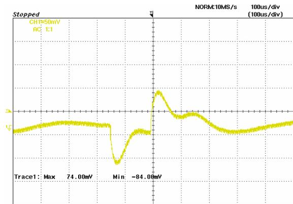
**Figure 22:** Typical transient response to step load change at  $10A/\mu S$  from 50% to 75% and 75% to 50 of  $I_o$ , max at 12Vin, 3.3V out
