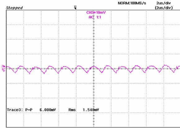
Figure 7: Output ripple & noise at 12Vin, 0.9V/50A out
