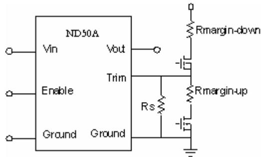
**Figure 29:** Circuit configuration for output voltage margining
