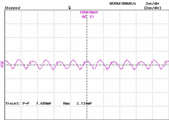
Figure 9: Output ripple & noise at 12Vin, 1.5V/50A out
