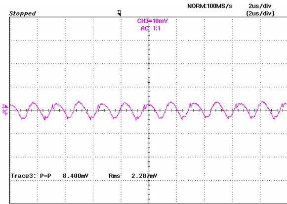
Figure 10: Output ripple & noise at 12Vin, 1.8V/50A out
