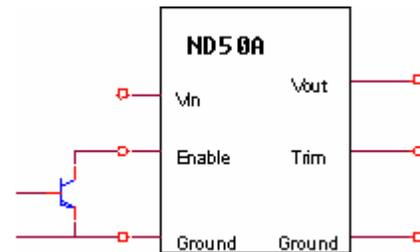
Figure 23: Enable Input drive circuit for ND series
