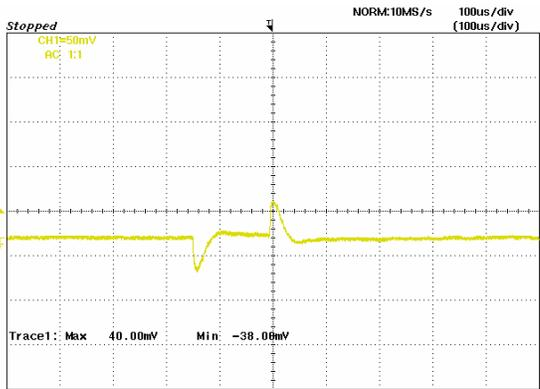
**Figure 17:** Typical transient response to step load change at 10A/μS from 50% to 75% and 75% to 50 of Io, max at 12Vin, 0.9V out
