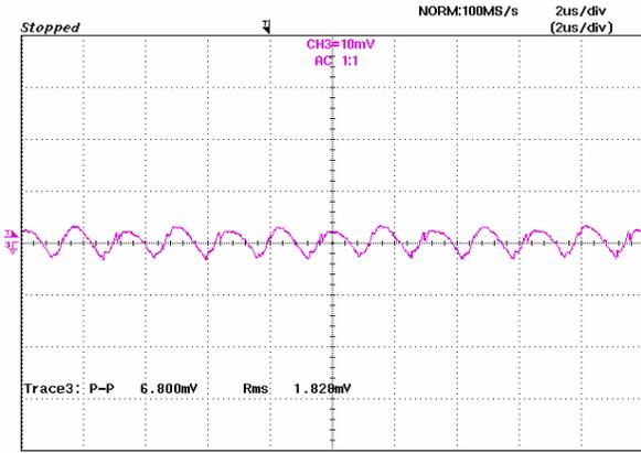
Figure 8: Output ripple & noise at 12Vin, 1.2V/50A out
