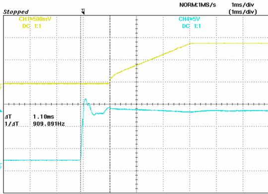
**Figure 13:** Turn on delay time at 12Vin, 0.9V/50A out
