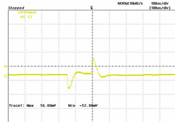
**Figure 18:** Typical transient response to step load change at 10A/μS from 50% to 75% and 75% to 50 of Io, max at 12Vin, 1.2V out
