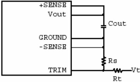
**Figure 28:** output voltage trim with voltage source
