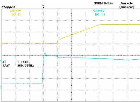
**Figure 15:** Turn on delay time at 12Vin, 3.3V/50A out
