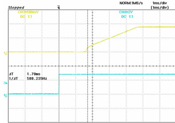
**Figure 14:** Turn on delay time Remote On/Off, 0.9V/50A out
