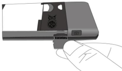
**To remove the micro-SD card**, press the card to release it.
