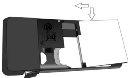
5. As shown, insert the back cover from the bottom. Push the cover until it is locked.
