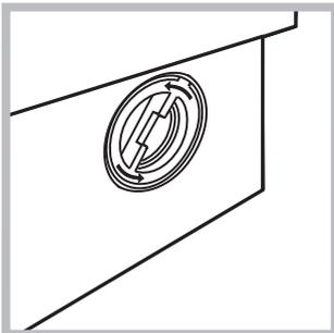
1. unscrew the lid rotating it anti-clockwise (see figure): a little water may trickle out. This is perfectly normal;
