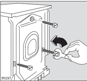
1. Unscrew and remove the three rear screws by means of a key.
