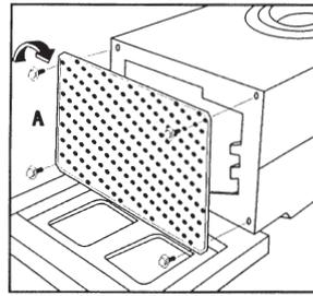
4. Unscrew and remove the four feet. Fit the grid on the bottom of the machine and re-fit the four feet. Tighten up the lock nuts on all feet.
