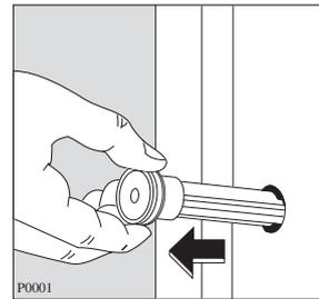
5. Place the machine in an upright position and remove the three plastic bolts.
