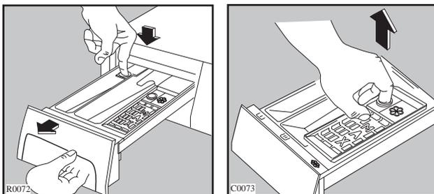
Detergent can also accumulate inside the drawer recess: clean it with an old toothbrush. Refit the drawer after cleaning.
