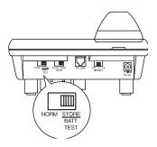
If the BATT TEST indicator does not light or is dim, replace the batteries.
