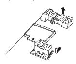
Plug one end of the supplied short modular cord into the TEL LINE jack on the back of the phone and plug the other end into a modular phone line jack. Then align the base's keyhole slots with the wall plate studs (or screws) and slide the base downward to secure it.
