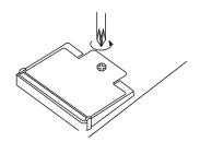
2. Put the batteries into the compartment as indicated by the polarity symbols (+ and –) marked inside.
