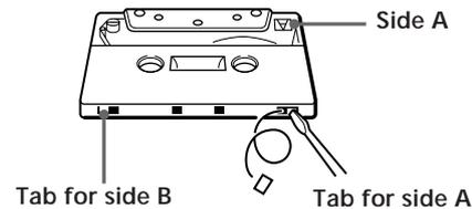
To record on a tape with a missing record-protect tab
