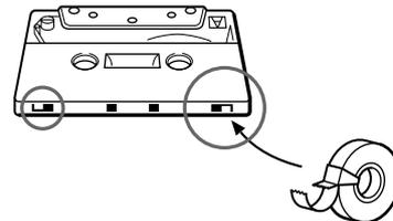
When you are using a type II or type IV tape, be careful not to cover the detector slots that the deck uses to determine the tape type.
