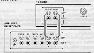
The illustration shows how the input and output terminals should be properly hooked up via the interconnect cords supplied with the unit to the Tape input and output terminals of your amplifier ( integrated amplifier, preamplifier or receiver ).
