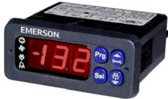
The EC2-352 is a dedicated refrigeration controller with superheat and a driver for an Alco Controls Electric Control Valve EX2. In addition the EC2-352 controls air temperature and manages defrost and fan(s).
