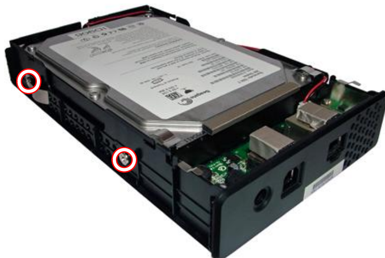
Fig. 3 Removing the hard disk drive screws.
