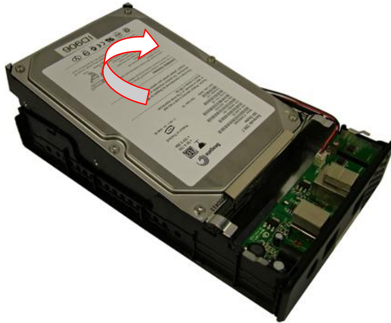
Fig. 4 Removing the hard disk drive.
