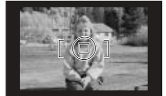
**7. When the focus signal appears in the viewfinder, press the shutter-release button all the way down to take the picture (p. 28).**
