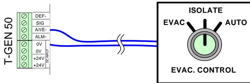
**Figure 5-6. Wiring an Evacuation Controller to a T-Gen 50**
