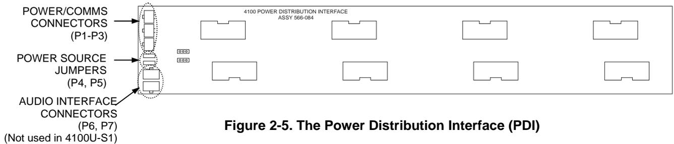
**Figure 2-5. The Power Distribution Interface (PDI)**
