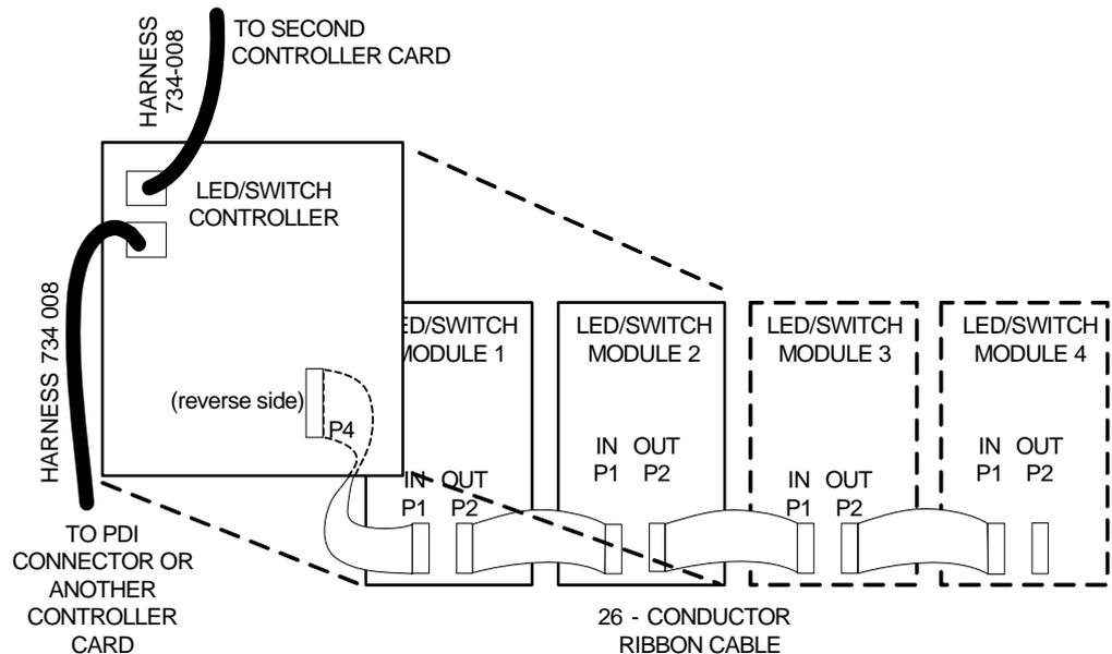
**Figure 2-15. LED/Switch Controller Wiring**
