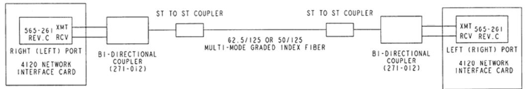
**Figure 3-7. Coupler Wiring**
