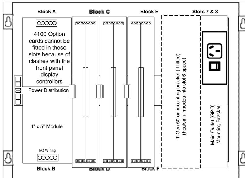
Up to four 2" x 11 1/2" motherboards can be mounted in the expansion bay. Three motherboards fit into Slots 3 through 5; the fourth can be added in Slot 6 if a T-Gen 50 is not fitted.
