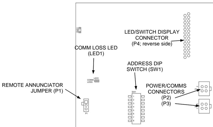
**Figure 2-12. LED/Switch Controller**
