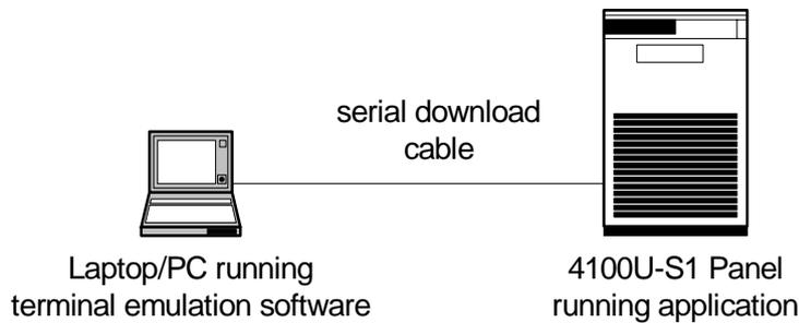
**Figure 7-1. Service and Diagnostic Interface**
