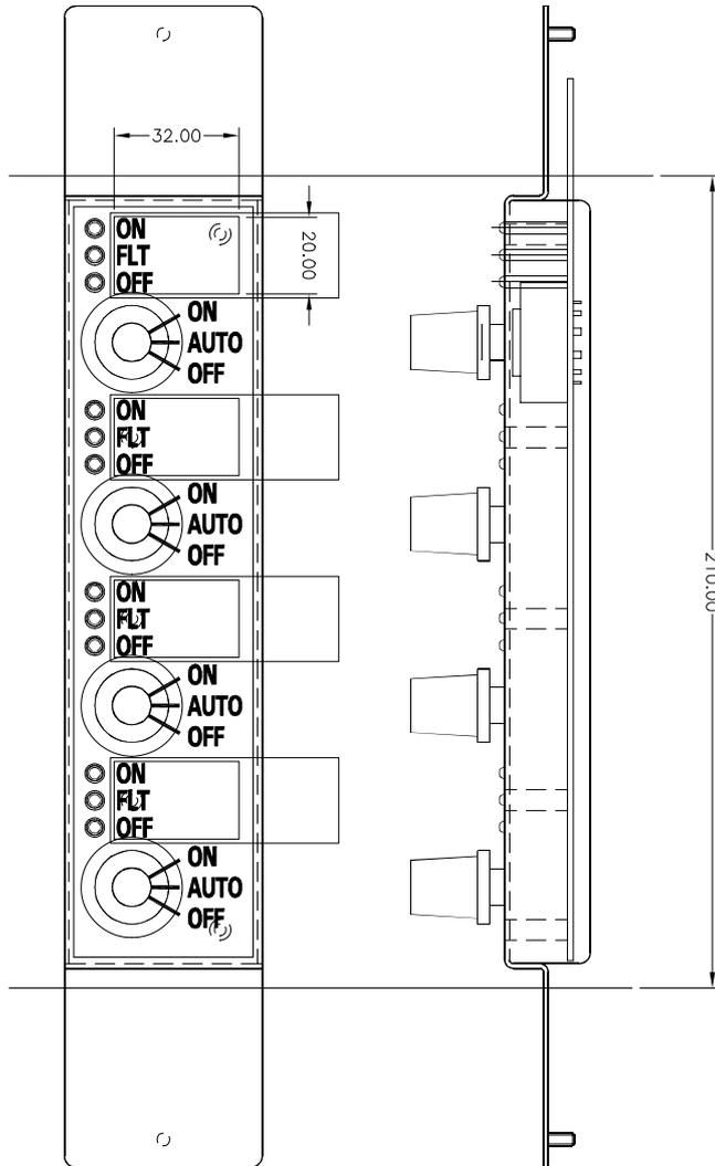
Figure 2-16. ME0456 Fan Control Module
