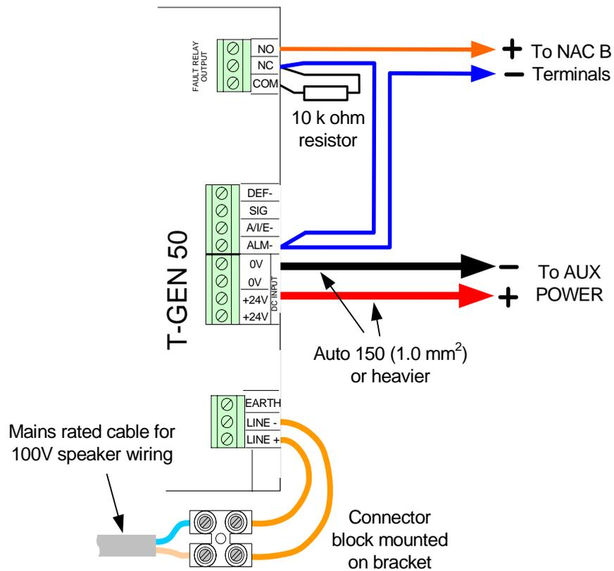
Figure 5-5. NAC Connection to a T-Gen 50
