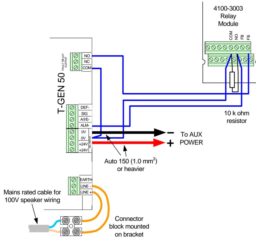
**Figure 5-4. Relay Module Connection to a T-Gen 50**
