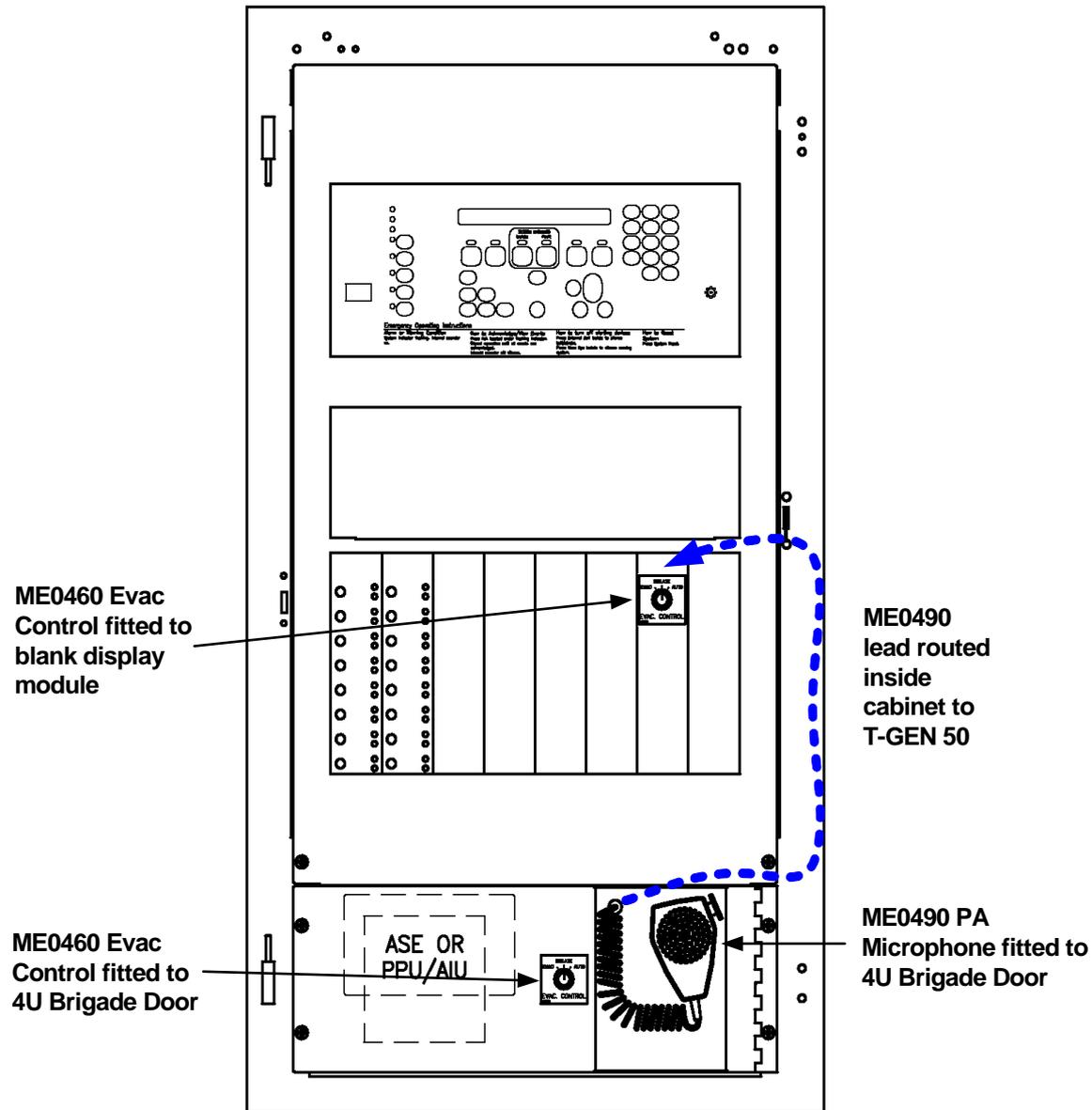
Figure 5-7. Examples of Evacuation Controls and PA Microphone
