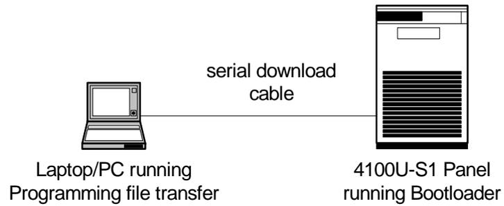
**Figure 7-3. Bootloader Interface**
