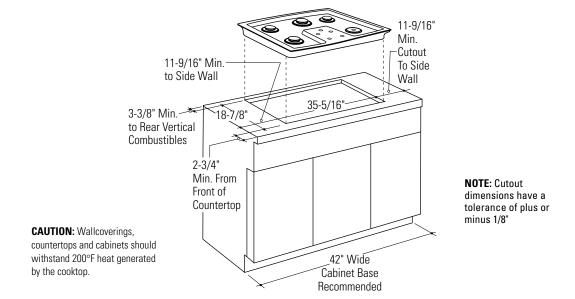
Measure carefully when cutting countertop. Make sure sides of opening are parallel and rear and front cuts are exactly perpendicular to sides.
