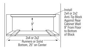
**NOTE:** The support must be level, rigidly mounted and capable of supporting 150 lbs.
