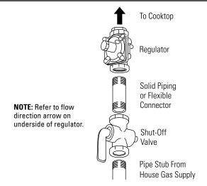
**IMPORTANT:** Disconnect the cooktop and the individual shut-off valve from the gas supply piping system during any pressure testing of that system at test pressures greater than 1/2 psig. Isolate the cooktop from the gas supply piping system by closing the individual manual shut-off valve to the cooktop during any pressure testing of the gas supply piping system at test pressures equal to or less than 1/2 psig.
