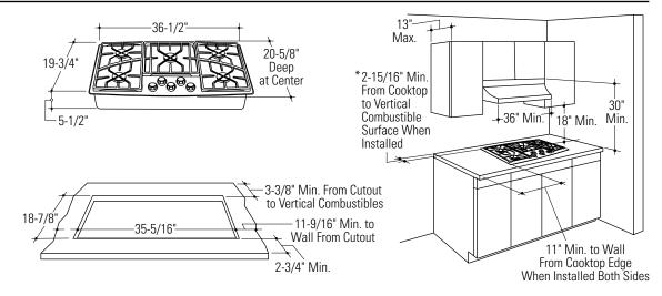
\* If a countertop backsplash is used, it must be constructed of non-combustible materials (such as masonry, ceramic, granite, stainless steel, etc.) whenever the cutout to rear vertical surface is less than 3-3/8".
