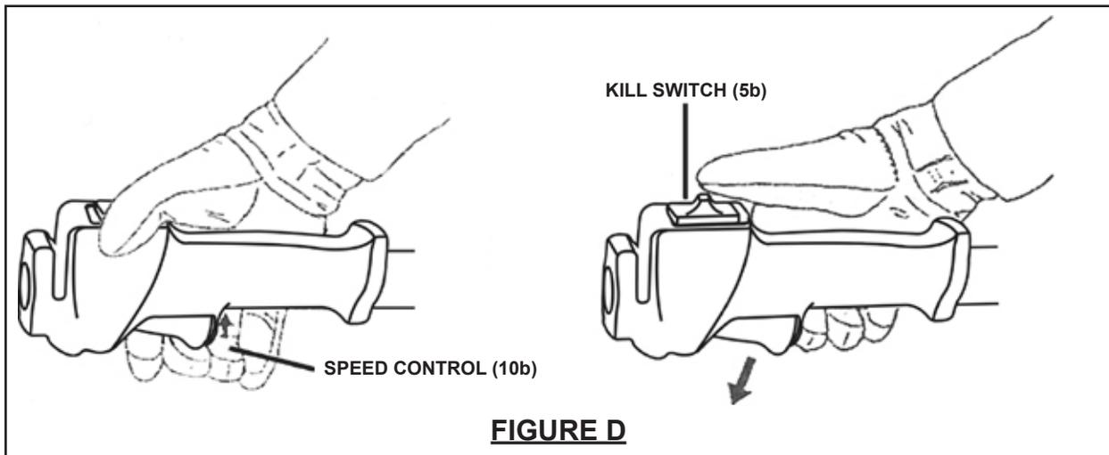
10. As soon as the Engine is running, check to make sure the Choke (76) is in its open position. Squeeze the Speed Control (10b) briefly and let up. The Speed Control will revert to its original position, causing the Engine to idle. **(See Figures C and D.)**
