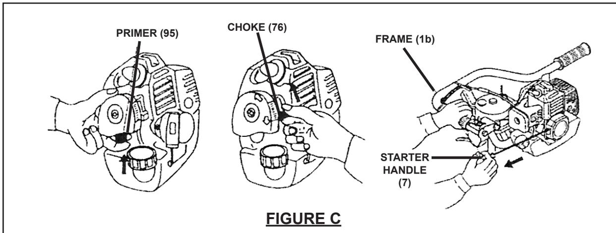
3. Depress the Primer (95) three to four times. **(See Figure C.)**
