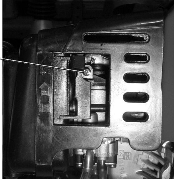
7. Once the Engine is started, set the Choke (76) to its open position.
