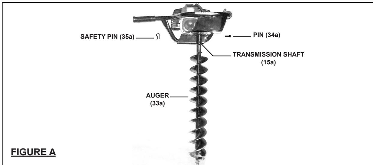
Insert the shank of the Auger (33a) fully upward into the Transmission Shaft (15a). Align the mounting holes in the Auger and Transmission Shaft. Then secure the Auger to the Auger Drill, using the Pin (34a) and Safety Pin (35a).
