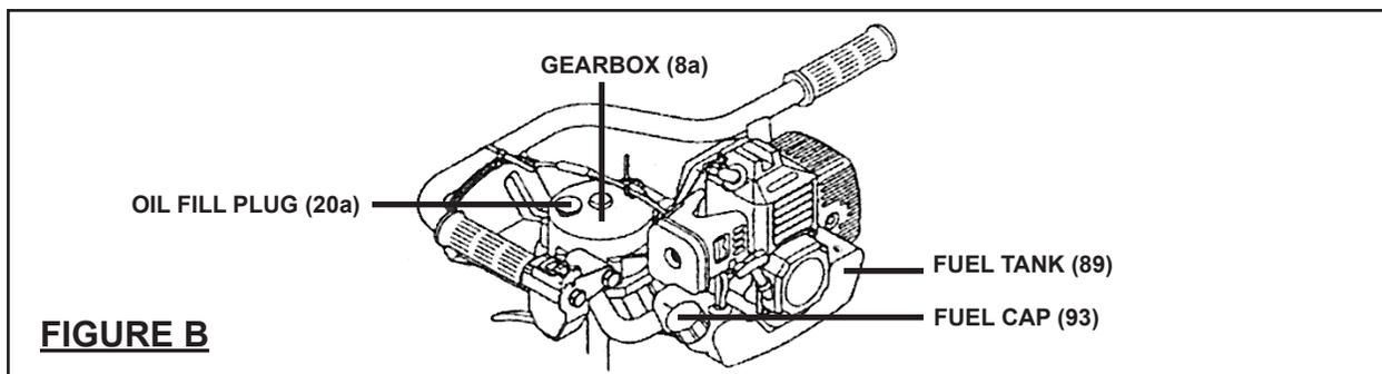
3. Once the proper fuel mix is obtained, remove the Fuel Cap (93). Fill the Fuel Tank (89) approximately 3/4 full with the fuel mix. Then, replace the Fuel Cap. (See Figure B.)
