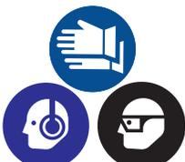
**Always wear safety equipment.** When operating the Auger Drill, always wear ANSI-approved safety impact eye goggles, hearing protection, heavy duty work gloves, sturdy steel-toed work boots, and head protection.
