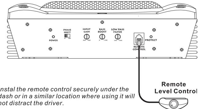
*Install the remote control securely under the dash or in a similar location where using it will not distract the driver.*
