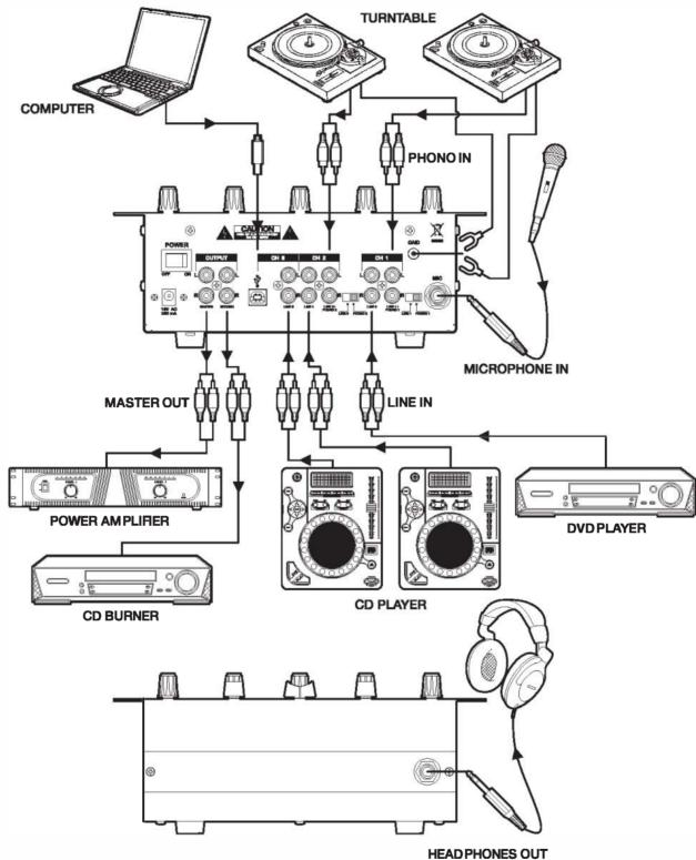
This mixer permits connection of up to seven (7) audio input sources, including one microphone. Such a system might include, for examples:
