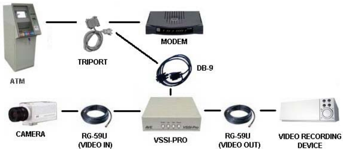
Figure 1: Typical VSSI-Pro Connections
