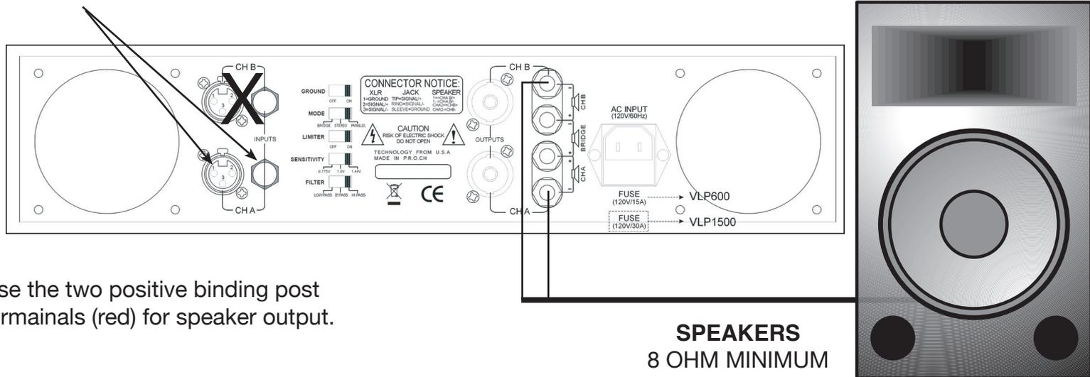
Use the two positive binding post terminals (red) for speaker output.
