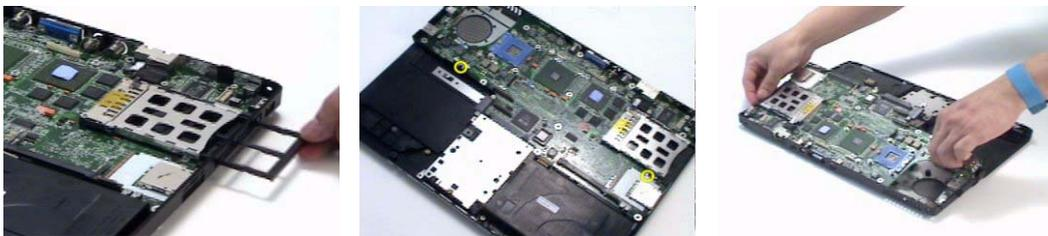
**IMPORTANT:**When assembling/disassembling the main board, whenever there is a mylar on the main board (see the highlighted with red below; the mylar is semi-transparent, film-like stuff ), it should be transferred “if necessary” to the replacement main board. Because the main board mylar should be stuck to the main board to prevent the antenna cable and the main board components short circuit. The short could cause the main board or the antenna cable burned.
