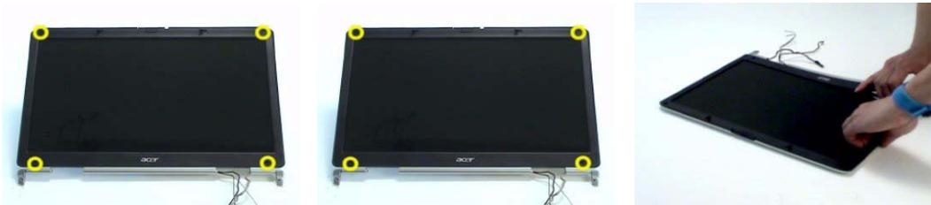
10. Remove the nine screws securing the LCD to the LCD panel.
