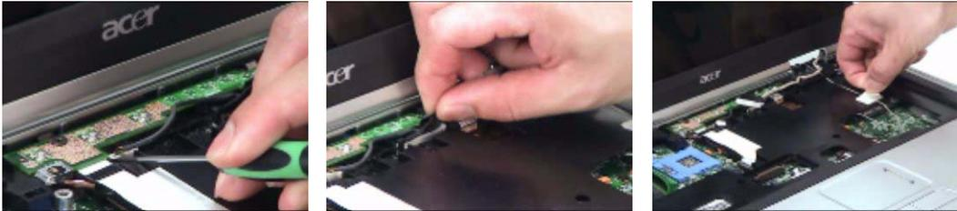
7. Remove the two screws securing the LCD module on the rear side.
