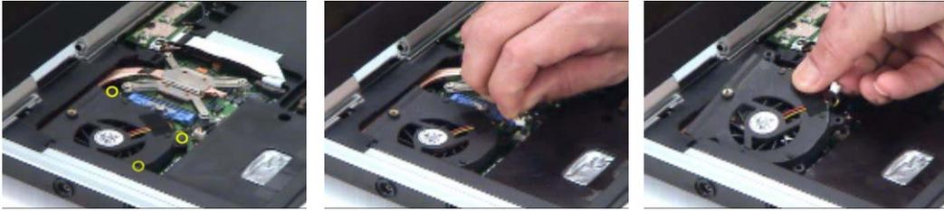
7. Remove the four screws securing the CPU thermal module.
