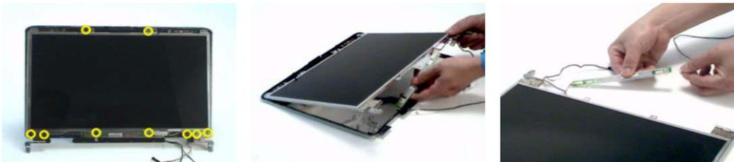
13. Disconnect the LCD inverter board.
