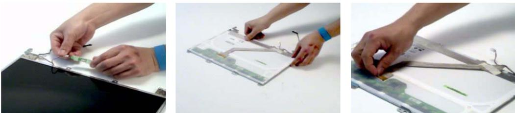
16. Remove the four screws securing the right LCD bracket, then remove the right bracket.
