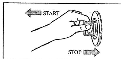
⑤ Pull Cycle Selector knob out to start the washer. If you wish to change setting after washer has started, push Cycle Selector knob in to stop the washer and reset to the new position. Setting can be changed at any time.
