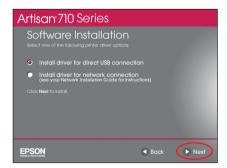
When prompted, connect a USB cable. Use any open USB port on your computer. Make sure the Artisan 710 Series is securely connected and turned on.
