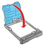
5 Squeeze the edge guides and slide them out. Then insert 4 x 6-inch or 5 x 7-inch photo paper with the glossy or printable side face-down.
