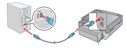
**Note:** If installation doesn't continue after a moment, make sure you securely connected the USB cable and turned on the Artisan 710 Series.
