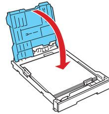
6 Squeeze the edge guides and slide them out. Then insert 4 x 6-inch or 5 x 7-inch photo paper with the glossy or printable side face-down.
