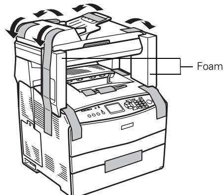
14. Place the CX11N/CX11NF in the original lower box housing.
