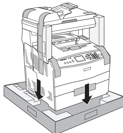
15. Attach foam to the top corners of the CX11N/CX11NF as shown below:
