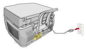
Plug the EPSON 1000 ICS into a grounded electrical outlet. Do not connect the USB cable yet.
