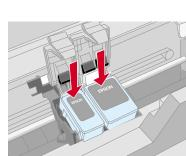
Press down the ink cartridge clamps until they snap shut.
