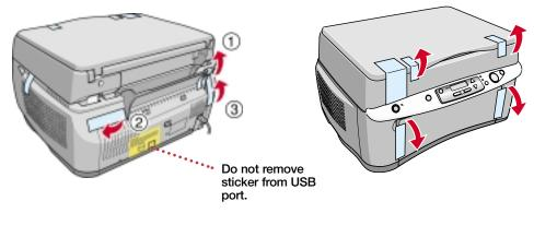
Note: There may be additional packing materials or tape in locations different from the ones shown in these illustrations. Do not remove the sticker covering the USB port.
