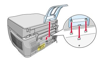
Insert the paper support into its three slots.
