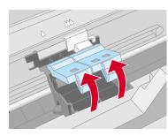
Insert the ink cartridges with the labels face-up.
