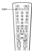
During playback, press DISP (Display). The elapsed time or the remaining time is displayed at the upper left. Each time you press DISP (Display), the display changes as follows:
