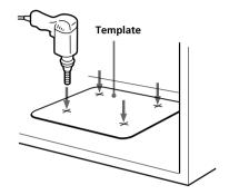
2 When the cabinet door overhangs the shelf and obstructs the unit, you can adjust the unit/shelf height.
