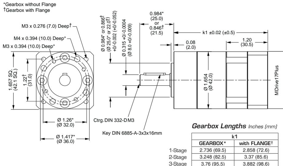
\*\*Include optional planetary gearbox by adding -G plus 3 characters to the end of an MDrive part number.
