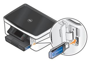
Bluetooth Dongle Connected appears on the display.
