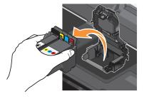
Warning—Potential Damage: Do not touch the printhead nozzles.
