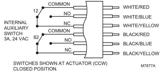
Fig. 7. ML6284 Actuator wiring for auxiliary switches.
