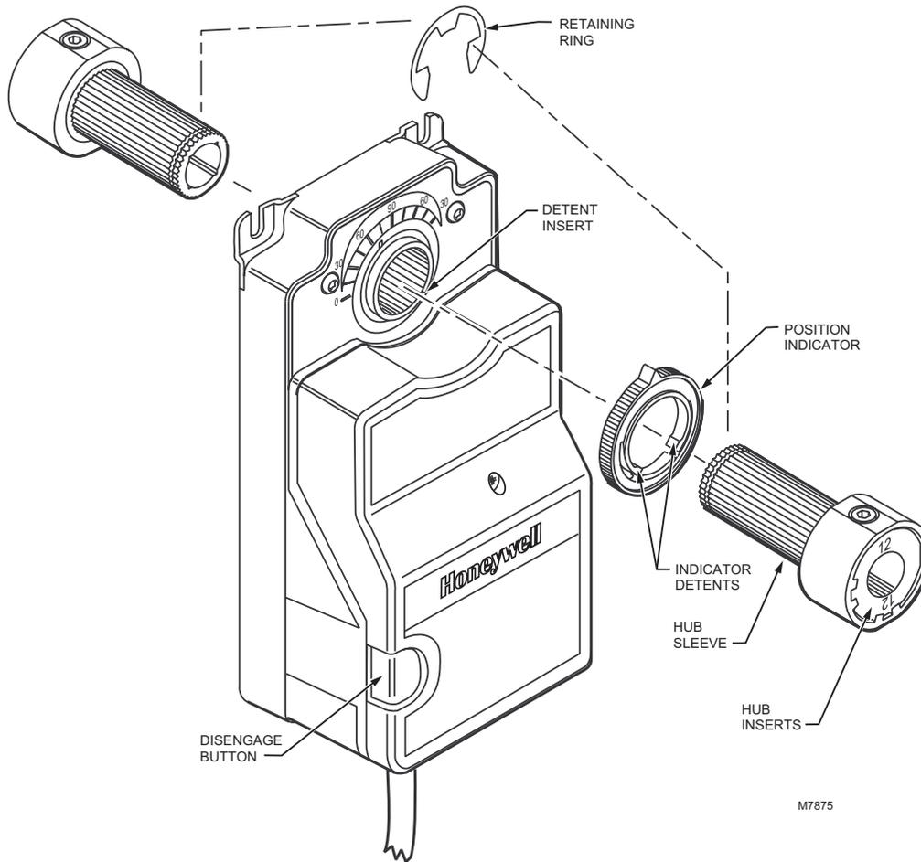
Fig. 3. Mounting hub to inside of actuator.
