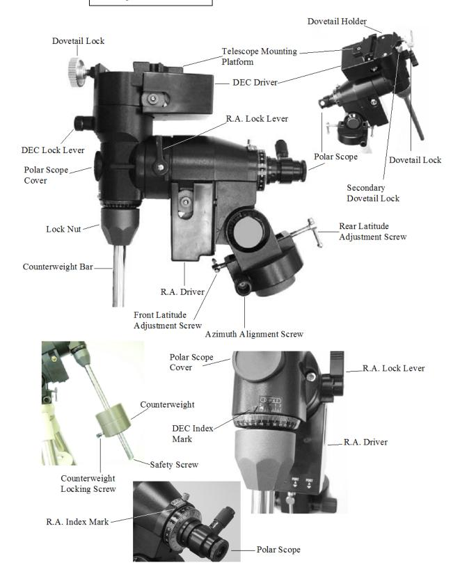
Since the fully assembled telescope can be quite heavy, position the mount so that the polar axis is pointing towards north before the OTA and counterweight are attached. This will make the polar alignment procedure easier.
