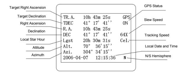
GPS status: When the power is turned on, it shows "GPS ON". When it finds the satellite and receives GPS signal, it shows "GPS OK".
