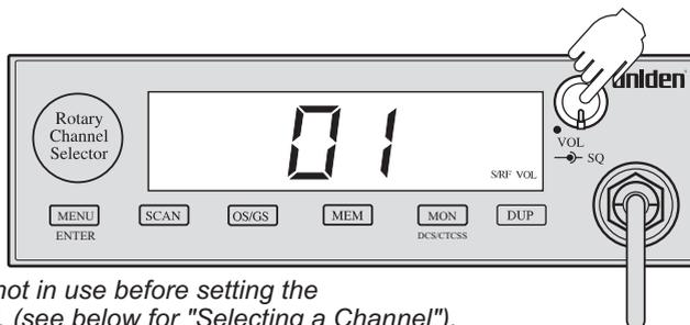
**NOTE** You must select a channel which is not in use before setting the SQUELCH control. (see below for "Selecting a Channel").
