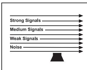
If you turn the Squelch fully counterclockwise it lowers the 'Squelch Gate' to the extent that all signals get through - weak, medium and strong signals and noise.
