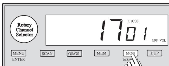
Turn the Rotary Channel Selector to select the desired CTCSS code 01 - 38. Press **MON** once to store the new setting. To turn off CTCSS (or DCS) select the oF code during setting.
