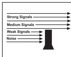
To set the 'Squelch Gate' to the desired level, turn the squelch knob counterclockwise until you hear noise. Then carefully turn the Squelch knob clockwise until the noise fades. Now only strong signals get through.
