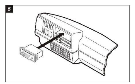
Re-connect the battery terminal and test the unit for proper operation. Snap the head unit/kit assembly into the sub-dash.
