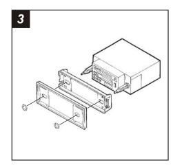
Attach the *Faceplate* to the *Snap-in Bracket*. Slide the aftermarket head unit into the kit and secure with shaft nuts.
