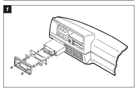
Disconnect the negative battery terminal to prevent an accidental short circuit. Remove the factory radio knobs and shaft nuts. Unclip the factory faceplate. Insert a flat-blade screwdriver into the shaft wells and push in on the side springs. Pull the factory radio out and disconnect the wiring.
