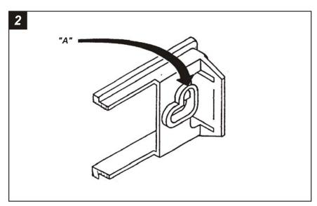
Slide the aftermarket head unit into the **Snap-in Bracket**. If the shafts of the head unit do not pass easily through the kit, cut and remove the upper-shaft tabs from the shaft openings. ("A")
