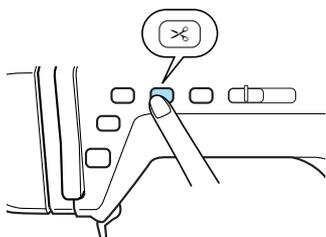
→ The needle automatically stops in the raised position, and the feed dogs are lowered.
