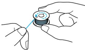
**4** Insert the wound bobbin into the bobbin case so that the thread unwinds in the direction of the arrow.
