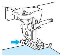
\* The presser foot remains level, enabling the fabric to be fed. Once the trouble spot has been sewn, the presser foot will return to its normal operation.
