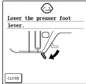
This message is displayed when the “Start/Stop” button, “Reverse/Reinforcement Stitch” button, “Thread Cutter” button or “Presser Foot Lifter” button is pressed while the presser foot lever is raised/the needle is lowered.
