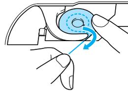
**6** After guiding the thread completely through the groove, pull it toward you to cut it with the cutter.
