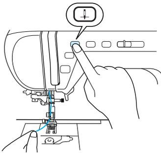
**4** Gently pull the upper thread to pull up the bobbin thread.
