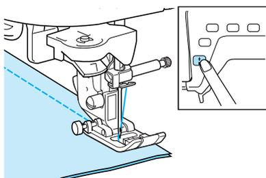
→ The machine stops with the needle in the fabric, and the presser foot is raised.
