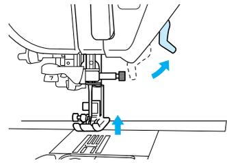
4 Press the black button on the presser foot holder to remove the presser foot.
