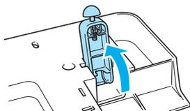
**2 Turn off the power and pull the flat bed attachment to the left.**
