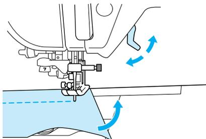
The pivot setting is useful when changing the sewing direction. When the machine is stopped at the corner of the fabric, the machine stops with the needle in the fabric and the presser foot is automatically raised so the fabric can easily be rotated (see "Pivoting" on page 47).
