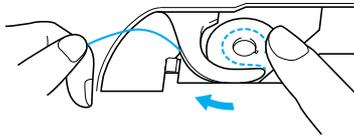
**3** While lightly holding the upper thread, press the “Needle Position” button twice to lower, then raise the needle.
