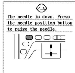
This message is displayed when the machine is turned on while the needle is lowered.
