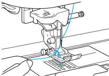
→ A loop of the bobbin thread comes out from the hole in the needle plate.
