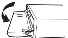
To close the front panel, press the left side until it locks as shown in the figure below.
