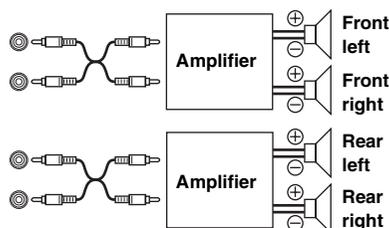
**Power IC ON :** The speakers are driven by the built-in amplifier.
