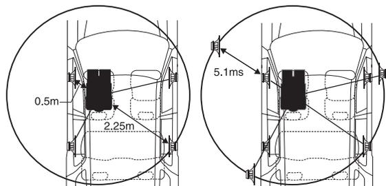
The sound is not balanced because the distance between the listening position and the various speakers is different. The difference in distance between the front left speaker and the rear right speaker is 1.75 m (68-7/8").
