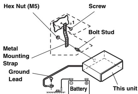
Reinforce the head unit with the metal mounting strap (not supplied). Secure the ground to a wire attached directly to the boat's negative battery terminal.
