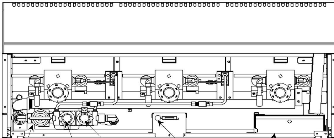
Main Shut-Off Valve      Left Pilot Button      Right Pilot Button (36" & 48" Models)      Spark Switch Button (Electronic Models)      Grease Drawer
