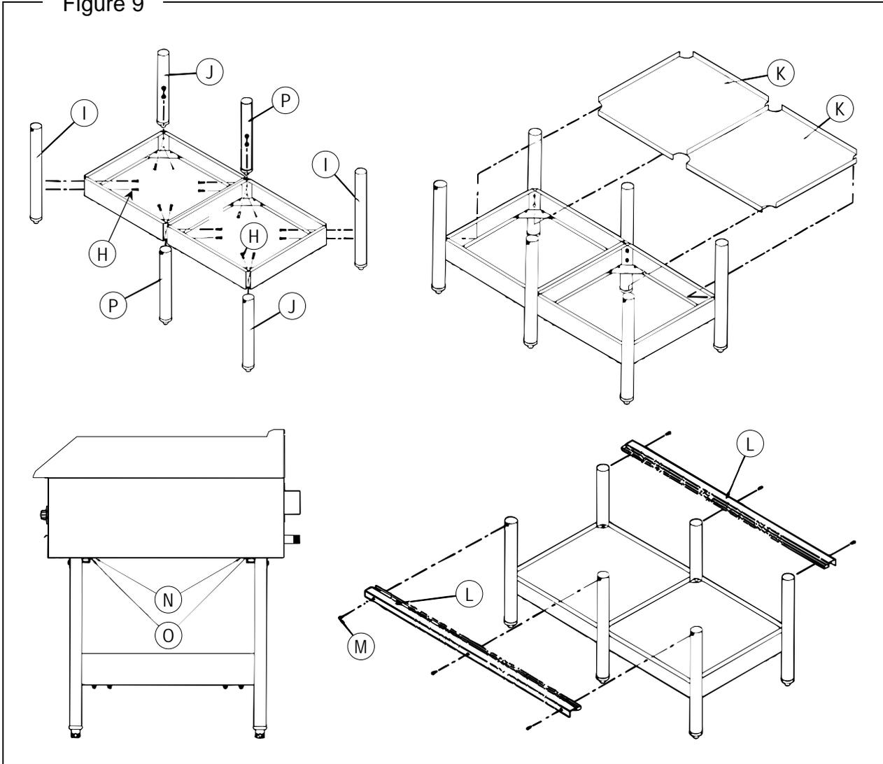
7. Check the partially assembled stand to make sure that the legs are straight and that all corners are square. Now tighten all bolts, but do not over tighten.
