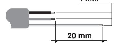
The end to be connected to the appliance must have an earth wire (yellow-green) at least 20 mm longer than the others.
