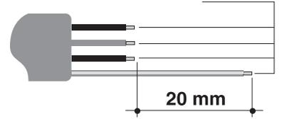
**2 - Operation at 220-240V~:** use a H05V2V2-F type three-core cable (3 x 4 mm<sup>2</sup> cable);
