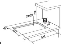
figure, to avoid damage from overheating. Make sure there is a minimum of 750 mm between the gas rings and any shelf that may be installed directly above them.
