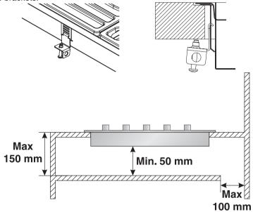
IMPORTANT: when installing the appliance above a cupboard, a dividing shelf, as shown above, must be installed.
