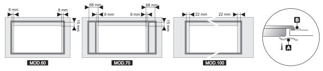
The diagram below shows the exact positions of the holes to be used for clamping the hob to the top correctly.
