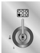
Each knob corresponds to the burner indicated. The appliance is equipped with an electronic lighting device. Just press and turn the knob anticlockwise to the maximum flame symbol  $\Delta$  until the burner lights. Keep the knob pressed for about 2 seconds to let the thermocouple heat up. If the burner turns off when the knob is released, it means that the thermocouple isn't hot enough. Repeat ignition and keep the knob pressed longer.
