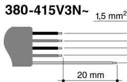
**For operation on 380-415V2N~:** use an H05RRR-F-type four-core cable (4 x 1.5 mm<sup>2</sup>).
