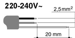
The cable end to be connected to the appliance must be provided with a ground wire (yellow-green) at least 20 mm longer.
