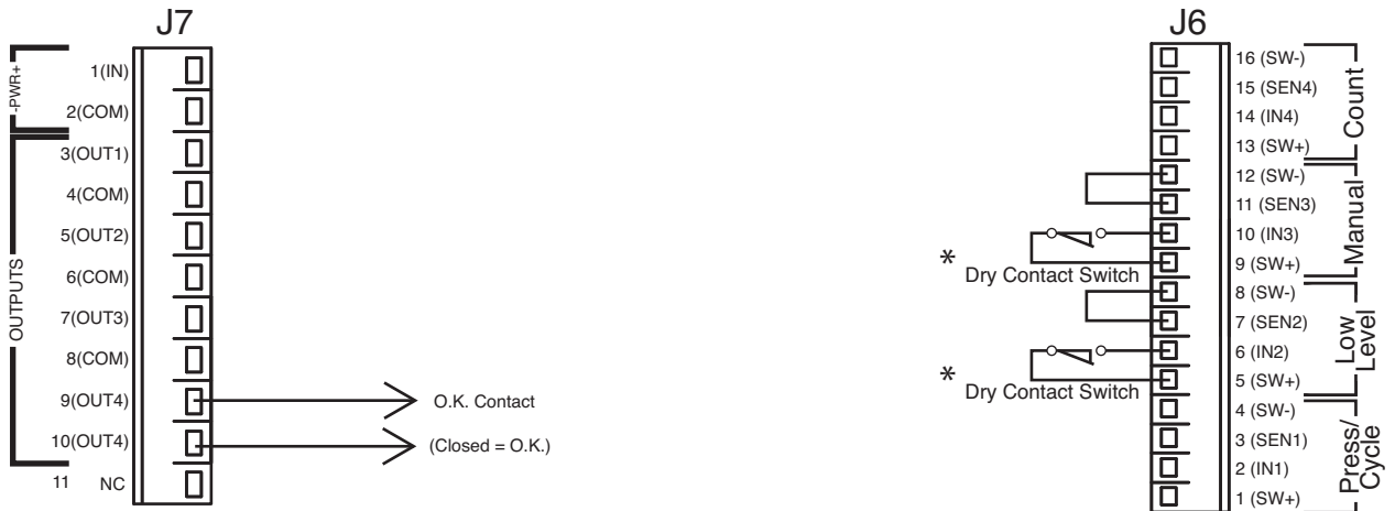
FIG. 17 Dry Contact, FIG. 8 shown. For other configuration, see FIG. 9 or FIG. 10.
