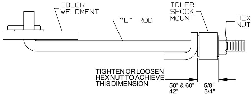
**NOTE:** Belt deflection or movement should be approximately 1/4" when measured at mid-point between pulleys.
