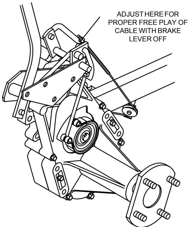
**NOTE:** Cable must have the recommended 1-1/2 to 2 inches of free play with parking brake released or drive belt may slip, causing loss of power.
