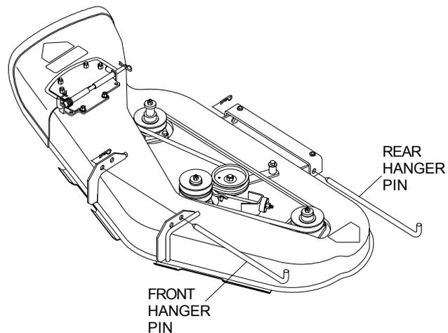
3. Slide deck from beneath chassis.
