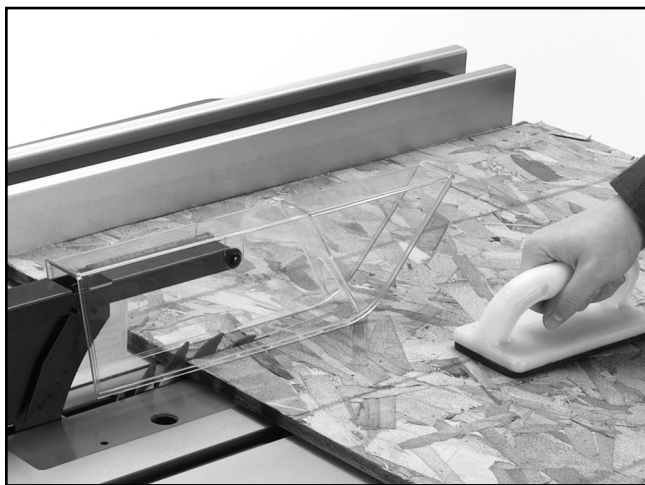
Figure 3. Push paddles being used to feed a work piece into the blade.
