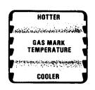
the oven is slightly hotter and the lower shelf slightly cooler. The base of the oven is quite a lot cooler. You can make use of these heat zones when you are cooking foods requiring different temperatures all at the same time.
