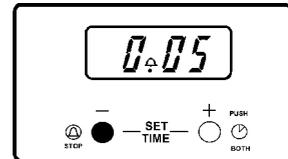
At the end of the timed period an alarm will sound. Switch off the alarm by pressing button 1.
