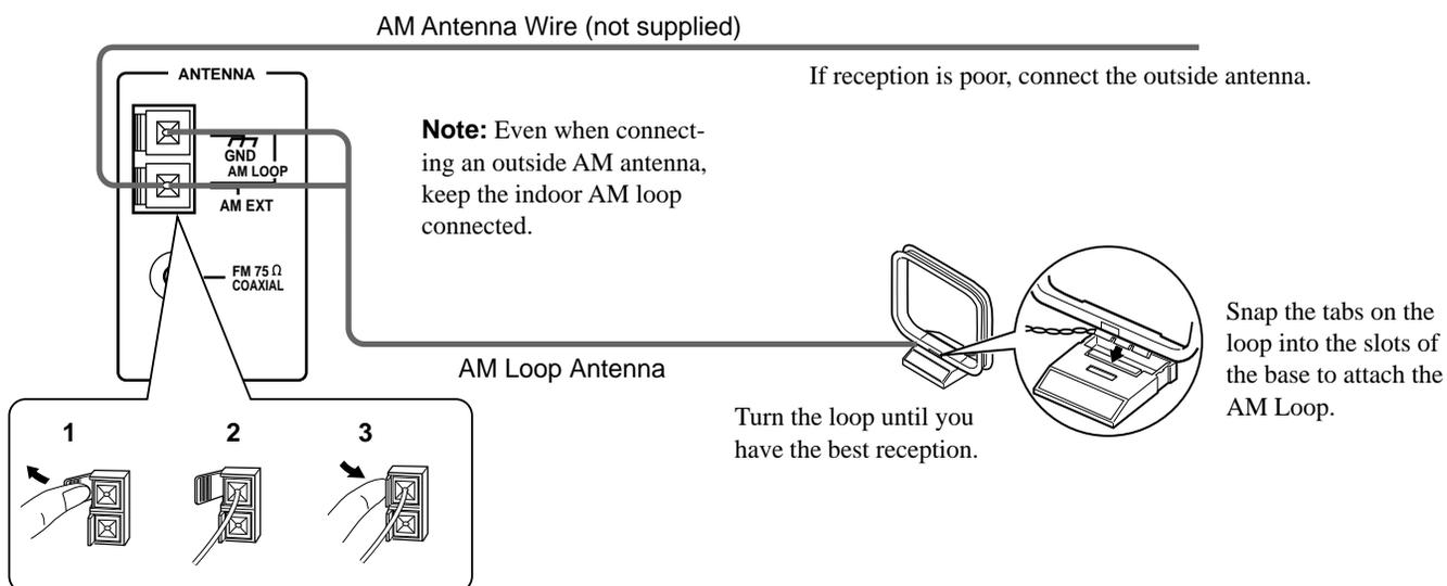
**CAUTION: Make all connections before plugging the Unit into an AC power outlet.**
