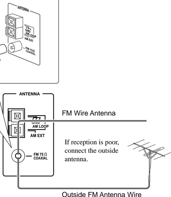
Before attaching a 75-ohm coaxial lead (the kind with a round wire going to an outside antenna), disconnect the supplied FM Wire Antenna.
