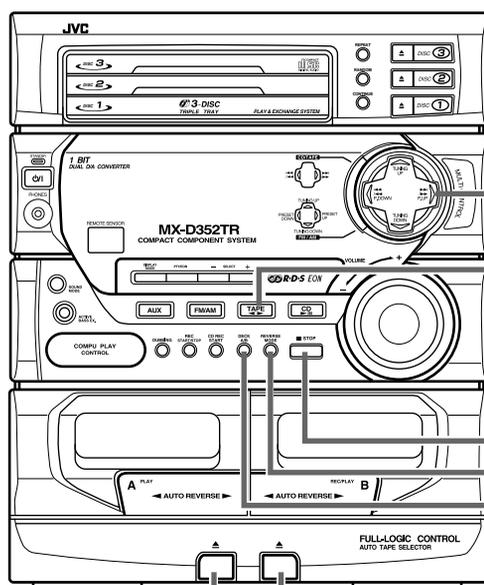
This illustration is of CA-D352TR. CA-D302T does not have the DISPLAY MODE, PTY/EON, and SELECT -, + buttons.
