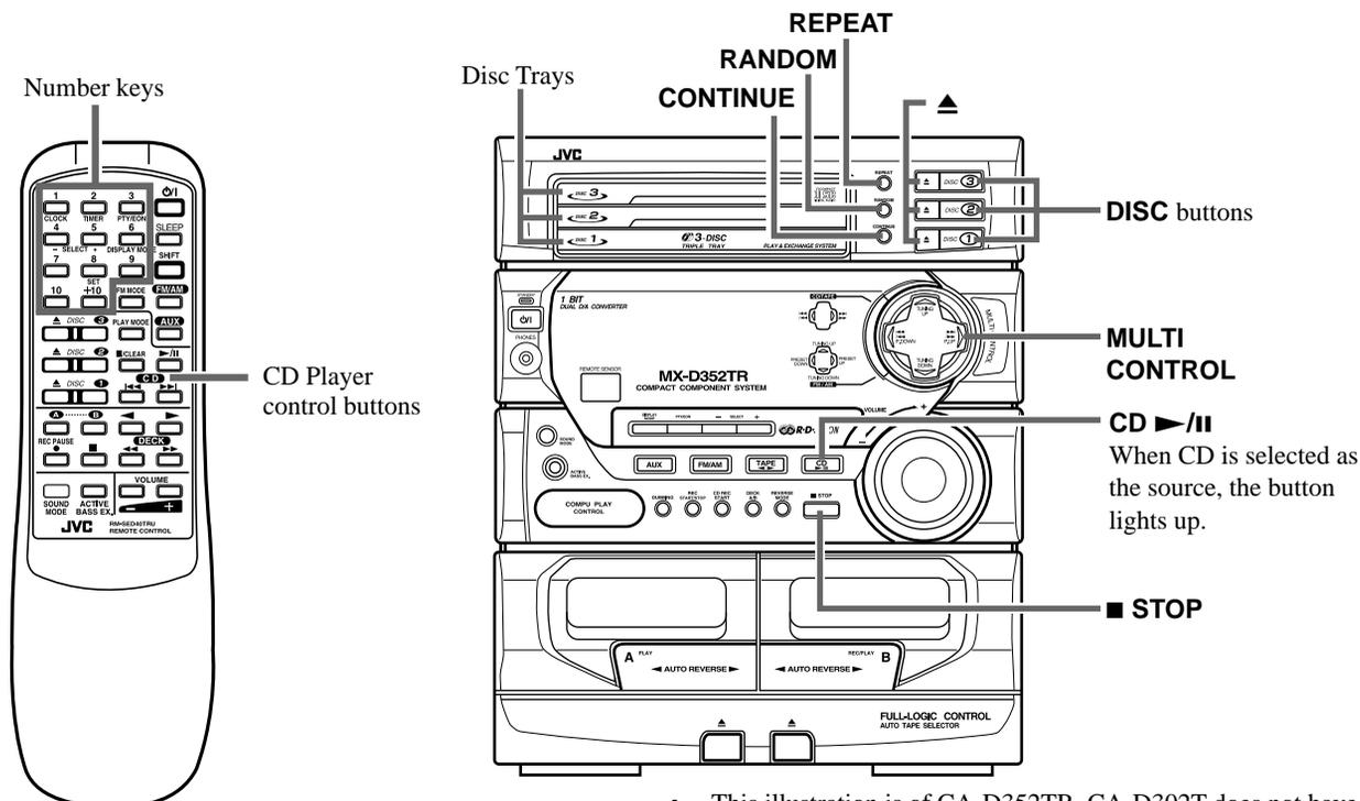
This illustration shows the Remote Control for CA-D352TR. The Remote Control for CA-D302T does not print the PTY/EON and DISPLAY MODE labels.
