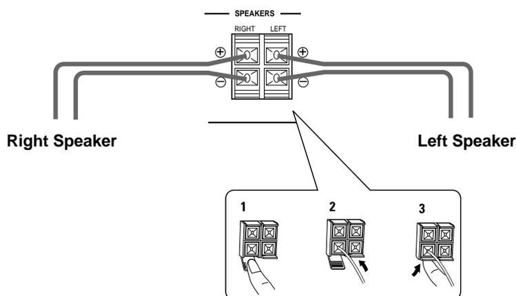
**IMPORTANT: Use speakers with the correct impedance only. The correct impedance is indicated on the back panel.**
