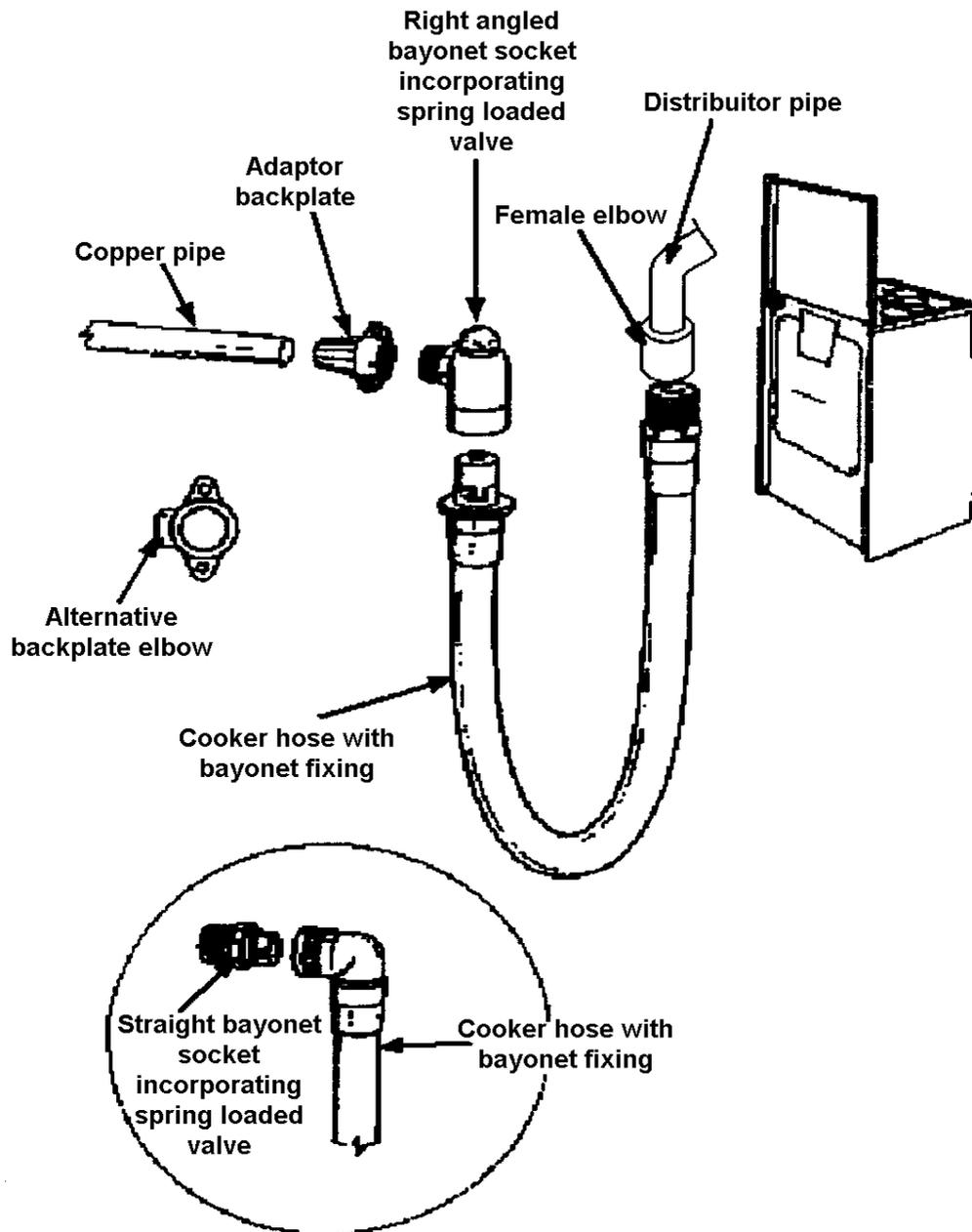
The appliance flexible connector should not be subjected to undue forces either in normal use or whilst connected or disconnected;
