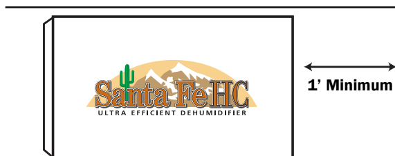
Figure 3: Installation requires a minimum 1' exhaust clearance.
