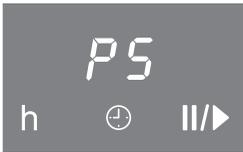
After selecting programming mode, **P** (Programme) and **5** (Status) will appear in the timer display. On hobs with 3 cooking zones, an additional indicator will appear at the rear left.
