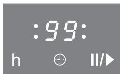
To set a time of more than 99 minutes, the timer must be set to hours (h). The time is then set in half hour stages. The half hour is indicated by a dot after the number.
